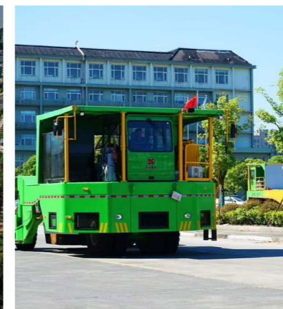
Unmanned Electric-Driven Slag Transport Truck
